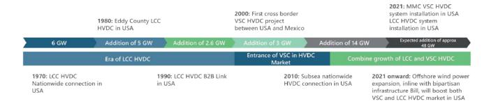
Fig 1: Timeline of deployment HVDC technology in the US. Source: Power Technology Research
