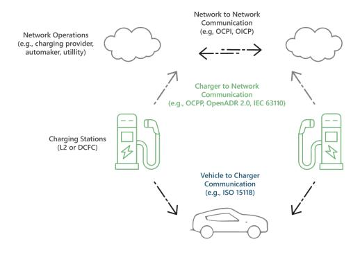
Figure 1: Different protocols used in EV charging.
